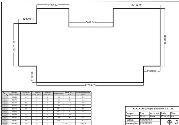
Use a building layout drawing with all lengths of the sides where Lucoline® should be installed to calculate the number of standard lengths, corners, cables and power supplies needed.
