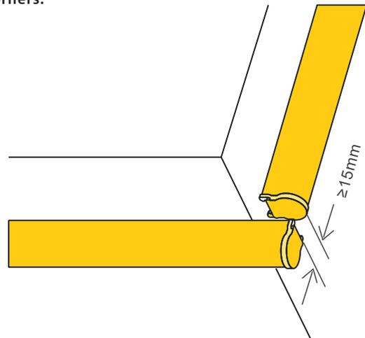
To install a corner on 2 sections these should overlap each other so that the end of the section is flush with the top of the other section. Again leave a gap as in the drawing to allow for thermal expansion. Snap the corner over the 2 sections to fix it.
