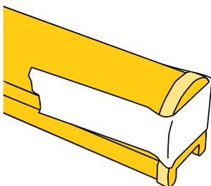
**5. Fix a tape to cure:** Put a piece of masking tape over the end cap and tube and let it cure for at least 20 minutes before handling it.
