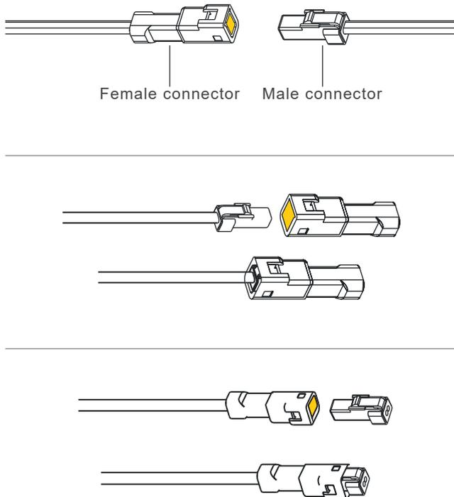
The JST connectors have a locking clip. Make sure these are fully engaged, making the connection IP67 water proof. Hide the connectors behind the tubes once connected. Do not pull or bend the cables too tight. This may damage the seal and compromise the IP rating.
