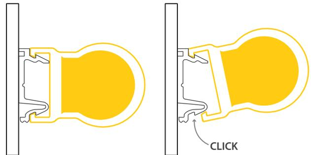
Hang the tube in the top side of all clips. Push the tube downward to snap it into the spring part of each clip. Check that the tube is secured in all clips, especially the Fixed Clip.
