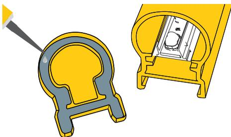
**4. Fix end cap:** Fill the edge of the cap with PMMA glue (Weldon 16, Acryfix or similar). Push it on the tube and hold for 30 seconds.
