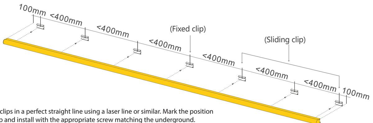
Install the clips in a perfect straight line using a laser line or similar. Mark the position of each clip and install with the appropriate screw matching the underground. Install one Fixed Clip in the middle of each section and all other at a maximum repeat distance of 400 mm. Install the last clips 100 mm from the end of the section. Install the clips with the arrows pointing up and the word TOP readable.
