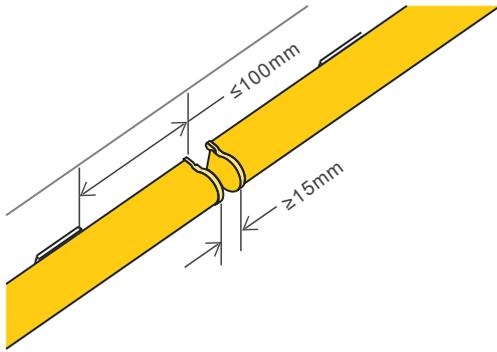
To allow for thermal expansion and contraction and to prevent damage the individual sections need to have a gap between them. Later covered with a joint cover.
