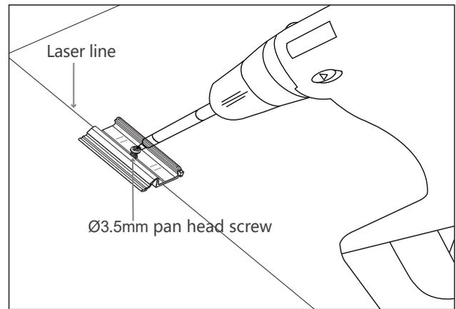
Use a laser line to mark the horizontal line on the building where the mounting clips should be installed. Per section install one Fixed Clip (L-CLIP-F) in the middle of the section to prevent it from moving on the building under temperature influences. Use Sliding Clips (L-CLIP-S) at a maximum repeat distance of 400 mm apart.
