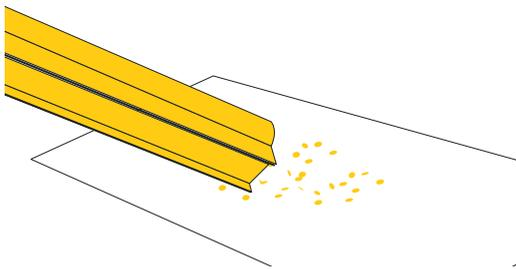
**2. Clean inside tube from plastic and aluminium residue.**
