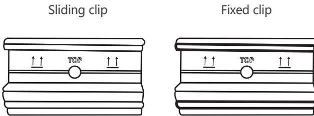
The Fixed Clip (L-CLIP-F) has rubber bands to prevent the tube from sliding. Only one should be used per section on a horizontal installation. In the case of a vertical installation use a Fixed Clip for every other clip to prevent the tube from sliding down under its own weight.
