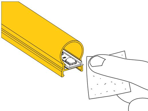
**3. Sand the edge:** Sand the edge of the tube & the PCB with the fine sand paper to ensure the edge is smoothed & uniform. Push back the PCB inside the tube.
