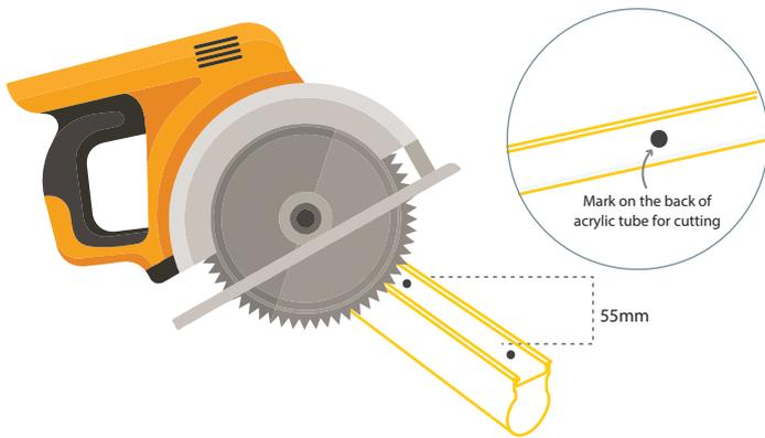
**1. Cutting of the tubes:** Locate the cutting positions (black dots) at the back of the tubes placed at every 55mm apart. Align the cutting position with the middle of the saw blade, place the tube flat on the platform, and cut the tube perpendicular to the saw blade. Please make sure that the saw blade is sharp to ensure that the cutting end face is smooth.
